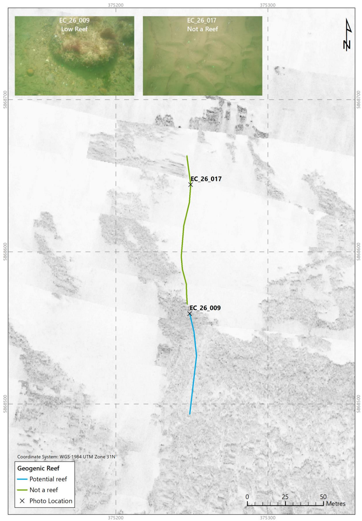
Figure 4.11: Potential geogenic reef (chalk) overlain on side scan sonar mosaic, transect EC_26
